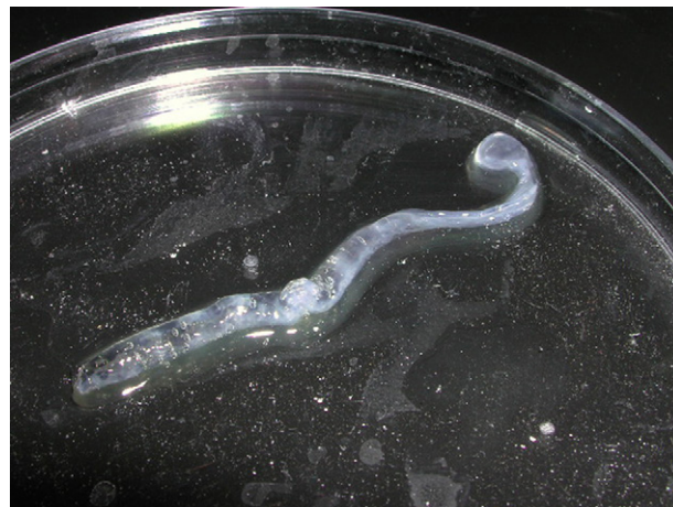
Fig. 7. The PVA-borax gel plug (1.5–3 mm in thickness) mechanically extracted from pig urethra and placed on a 9 cm (Ø) Petri dish.
